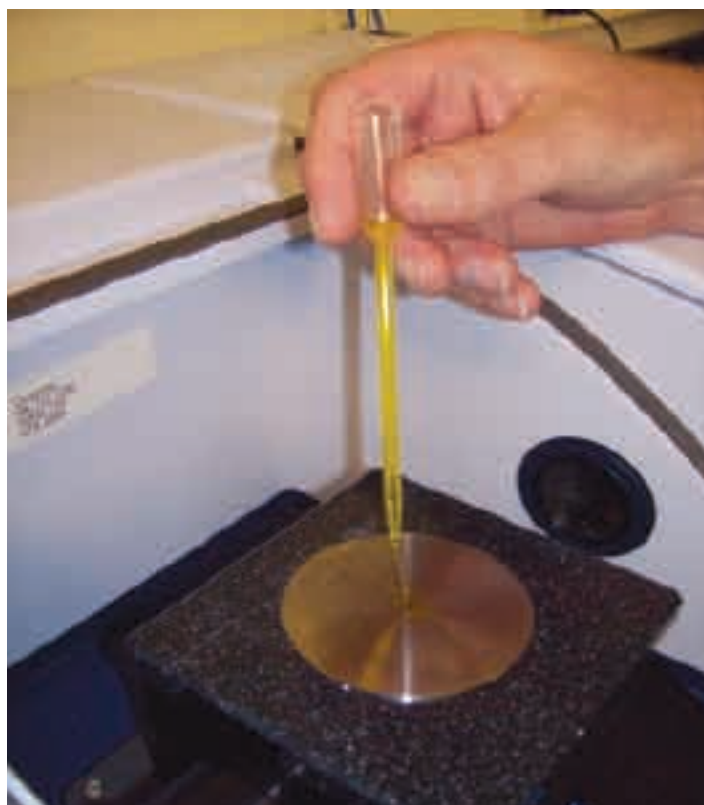
A drop of unprepared biodiesel is placed on a near infrared instrument to capture the quality traits for analysis
