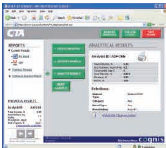
Quality measures can be viewed by plant personnel on a standard PC two minutes after the sample is taken
