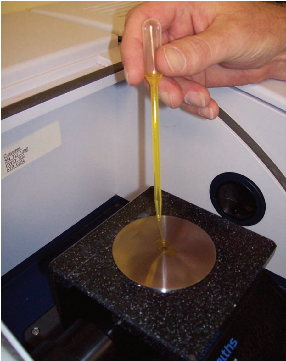
A drop of biodiesel is placed for analysis on the near infrared instrument.
